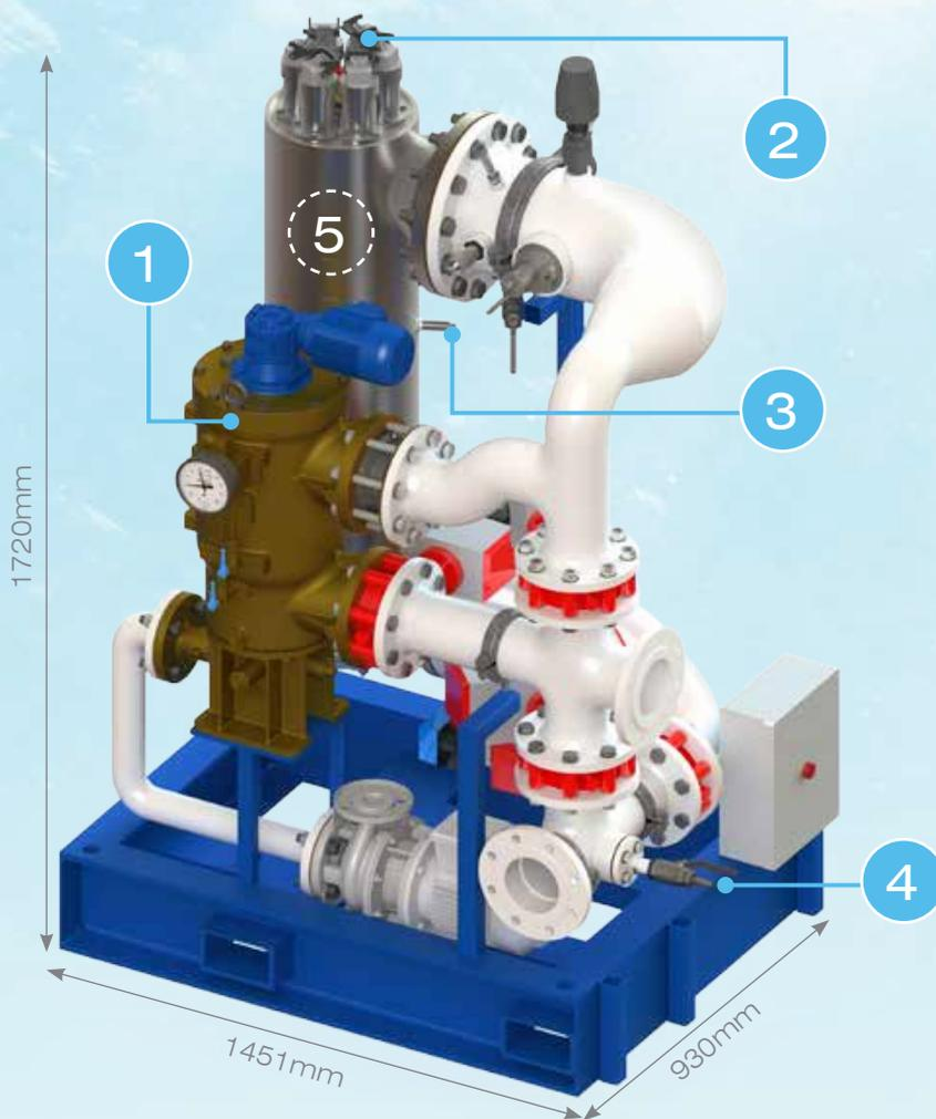
The Cathelco Evolution system is based on a combination of filtration and UV technology. It has been specifically designed for luxury yachts with a very compact filter, shorter UV chamber and very small overall footprint. Its capacity has been tailored to the needs of yachts and it is ideally suited to treat flow rates in the range of 34-135 cubic metres per hour.
