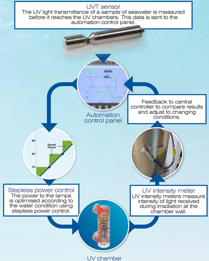
The unique Cathelco UVT sensor system has already proved its value in precisely adjusting the UV dose to changing water qualities. This is achieved by sampling sea water before it reaches the UV chamber and measuring the amount of UV light actually passing through it. This works in conjunction with UV intensity meters which are mounted on the chamber and measure the intensity of light which is received.
